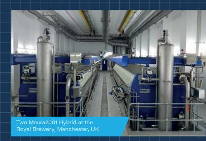
With the aim of reducing the oxygen pick-up in the filter a CO<sub>2</sub> injection was foreseen, leading in 2005 to the Meura2001 Carbo+. This filter was still composed with plates, made of 2 cloths or 2 membranes, installed alternately. Meura's research showed that sparging efficiency could be improved while filling all the chambers in the same direction. This led to the development of the unique chambers having one cloth and one membrane. The Meura2001 Hybrid was born in 2010.
