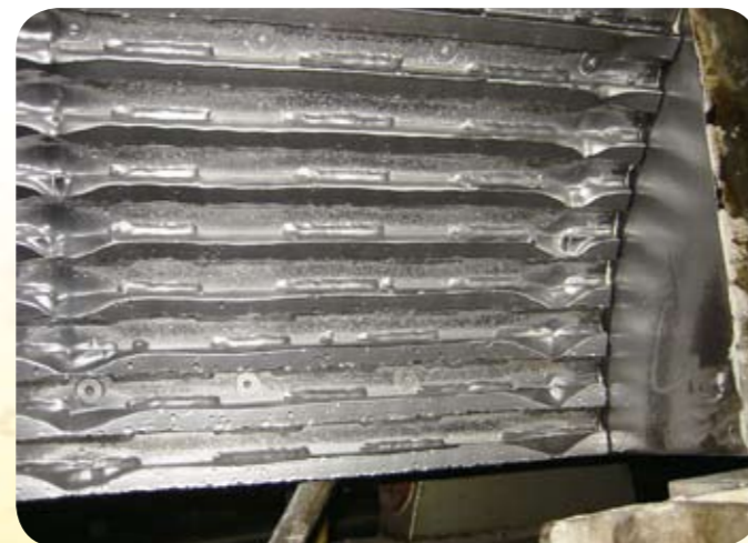
Example of a worn breaking plate showing that it is clearly protecting the sieves
