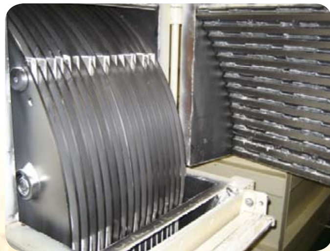
▲ Hammers and breaking plate of a CLASSICMILL
